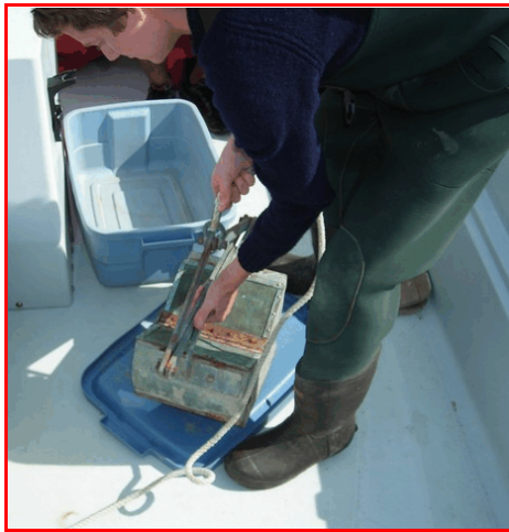
A-1. Benthic Ponar grab sampler being prepared for deployment.
