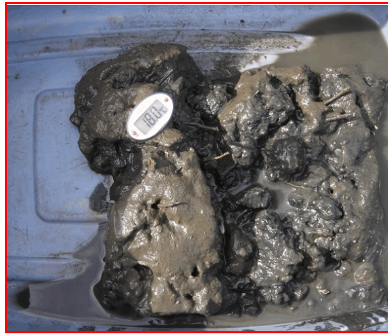
A-2. Example of sample obtain by grab sampler. Note worm tubes
